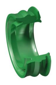
The newly developed, self-retaining EN seal-wiper ring for piston rods of pneumatic cylinders performs three functions: sealing, wiping and fixing. The EN profile consists of the known geometry of the EU profile with a double, flexible sealing lip plus a new
